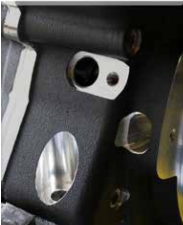
↑ The case and crank have been machined to accept stock Delphi style crank position sensors.
