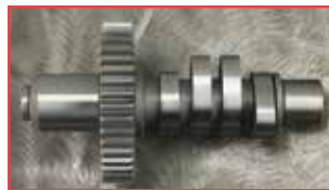
Knuckle cam. The two grinds made for this engine are described above.
