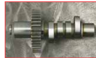
Cam for a 61 C.I. Pan engine. Because of the unusual cam design these engines don't run well with a "74" Pan cam so Andrews makes stock replacement "61" cams.
